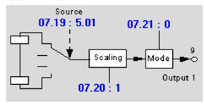
However, as stated above, this output will be positive in the forward direction and negative when operating in reverse.
