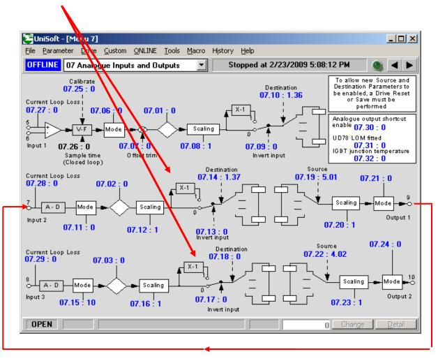
So.... if we take the bi-polar analog output from terminal 9 and wire it to either terminal 7 or 8 whichever is free, perhaps we could invert the signal depending on the direction bit #10.14.
