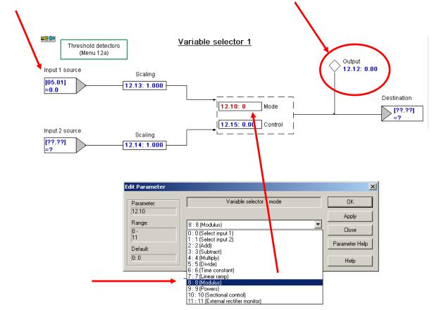
Now it is just a simple matter of assigning our analog output to this absolute value signal available at #12.12. For Unidrive SP and Commander GP20 the final assignment is shown below. (Don't forget to Store to make these assignments take effect and remain)
