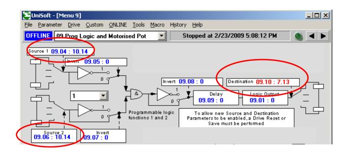
Now we just need an intermediate place to direct the result of the analog input that is being inverted. We could use one of the free registers up in Menu 18. I chose #18.11.
