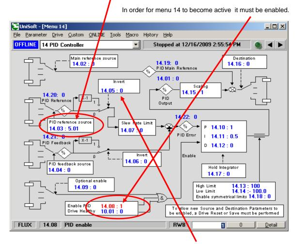
A similar philosophy that was used in Method 1 will be used here also that will change the inverter at #14.05 based on the direction bit #10.14.
