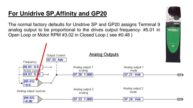
However, as stated above, this output will be positive in the forward direction and negative when operating in reverse.
